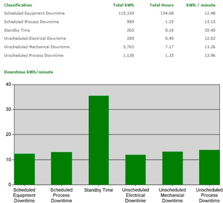
**Figure 11:** An example of tracking energy use during downtime - Schneider Electric Ampla Software
