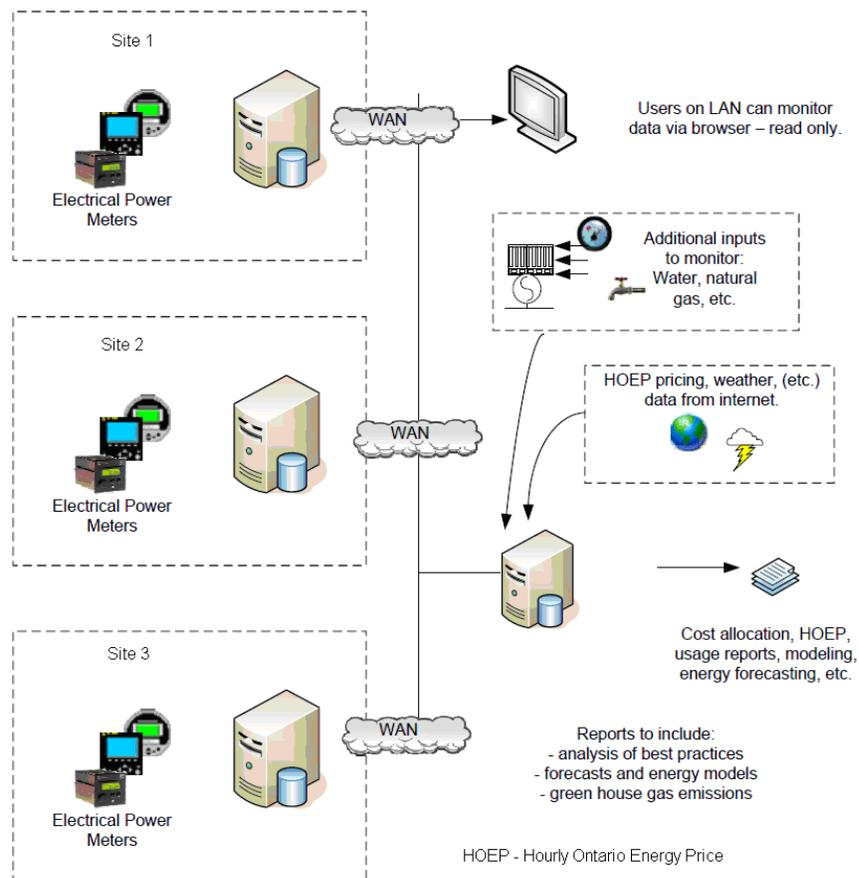
Figure 6: Real-time, multi-site energy tracking for an Ontario mining company (Schneider Electric)
