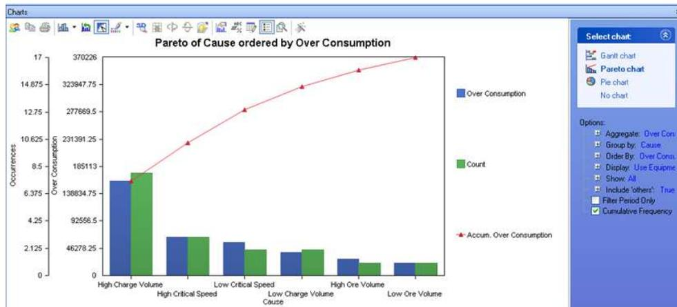
**Figure 12:** Energy “Overconsumption” Events - Schneider Electric Ampla Software
