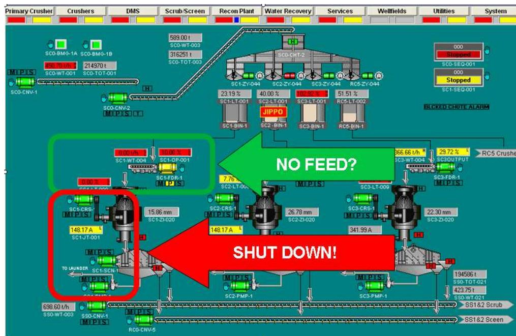
Figure 7: Automated contextual energy savings measures (Schneider Electric)
