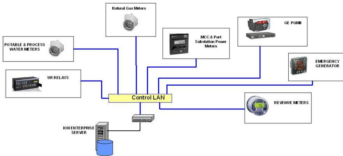
Figure 5: Site-wide energy tracking for an Ontario mining company (Schneider Electric)
